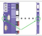
In order to prevent lateral movement from vibration and shock, both the **node module** and the **bus termination module** have an end clamp for firm attachment onto the top hat rail. Modules within the decentralized I/O island are then fixed with these clamps.
