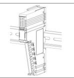
2. When connecting adjacent extension modules, make sure they are correctly mated together via the tongue and groove.
