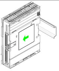
Remove the module from the DIN rail.
