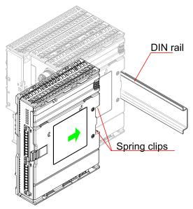
Align and insert the upper and lower guides on the left-hand side of the housing into the grooves of the adjacent module on the DIN rail. Push the module until the spring clips snap onto the DIN rail.
